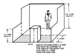
In-line Booths: Booths consist of 8-foot-high back drape and 4-foot-high side drape mounted on aluminum tubular frames. There is a 12-foot height limitation on in-line booths. Back of booth extending above the drape must be finished with no copy of any kind on it. Solid construction in excess of 4 feet in height must be a minimum of 5 feet back from the aisle to allow sight lines to adjacent booths.
